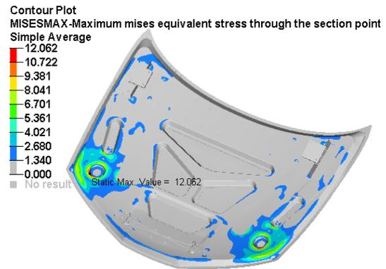
Fig. 10. Von-Mises stress Plot for Gravity load
