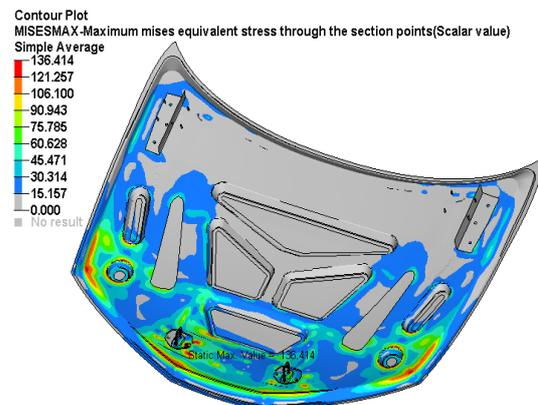
Fig. 12. Von-Mises stress Plot for Gravity load+ Latch Load
