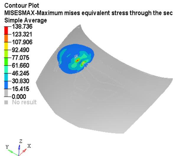
Fig. 28. Von-Mises stress Plot at Loc1
