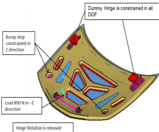
Fig. 6. Boundary Conditions for Latch Load Analysis
