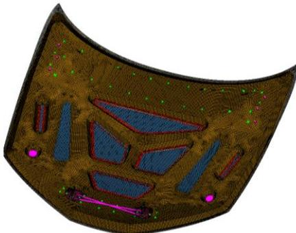
Fig. 2. Inner Hood Assembly FE Model
