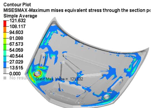
Fig 15 Von-Mises stress Plot Loading
