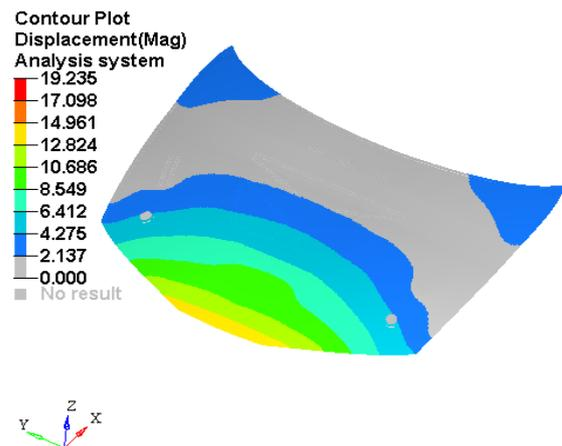
Fig. 11. Displacement Plot for Gravity + latch load
