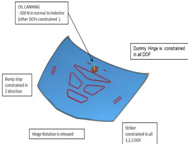
Fig8 Boundary Conditions for Oil canning Analysis
