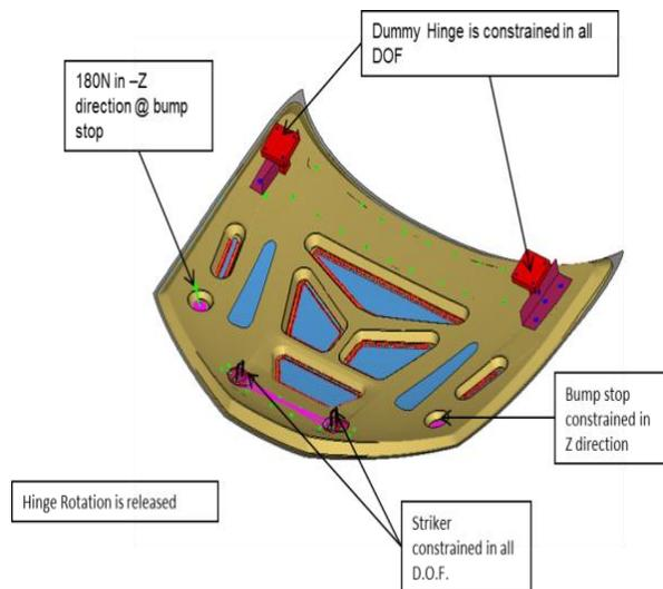
Fig. 4. Boundary Conditions for Torsional Rigidity Analysis
