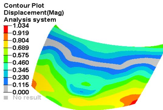
Fig. 25. Mode 4 at 64 Hz
