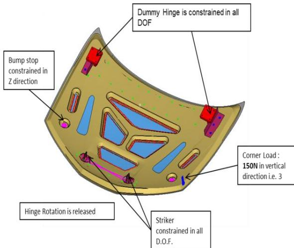
Fig 5 Boundary Conditions for Front Corner Stiffness Analysis
