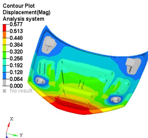
Fig. 9. Displacement Plot for Gravity load
