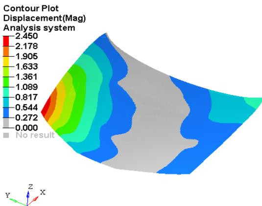
Fig. 19. Displacement Plot for gravity + loading step
