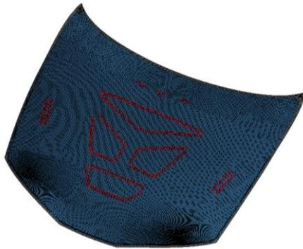
Fig. 1. Outer Hood Assembly FE Model
